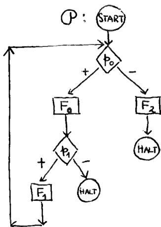
It is intuitively clear that, given an arbitrary machine  $M$ , this diagram allows us to generate for each  $x \in X$  at most one computation, obtained by following the "flow" of the diagram. We say that the diagram (a "syntactical" object) defines a program (a mathematical object.)
